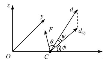
Figure 2: Catcher  $C$  applies force  $F$  to move in  $xy$ -plane. Unit vector  $d$ , parameterized by angles  $\phi$  and  $\psi$ , specifies the gaze direction. The catcher controls the **module of the force**  $F$  along with the **direction** of its application  $\theta$ , and **angular velocities**  $\omega_\phi$  and  $\omega_\psi$ .
