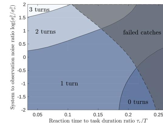
Figure 7: Switches between reactive and feedforward policies are determined by uncertainties and latency.
